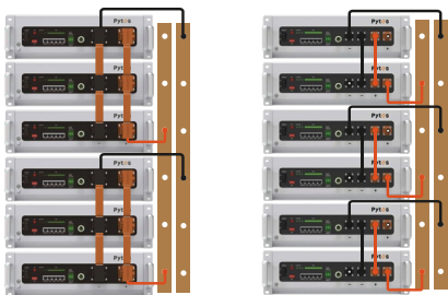
Figure 5-1 Schematic diagram of power cable connection
